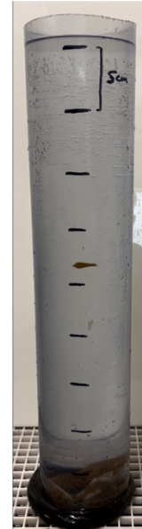
Figure 1. Picture of a vertical cylinder used for masticated kelp sinking rates.
